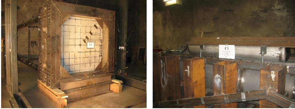
Figure 2. Experimental setup for test X1 (left) and projectile before the test (right).
