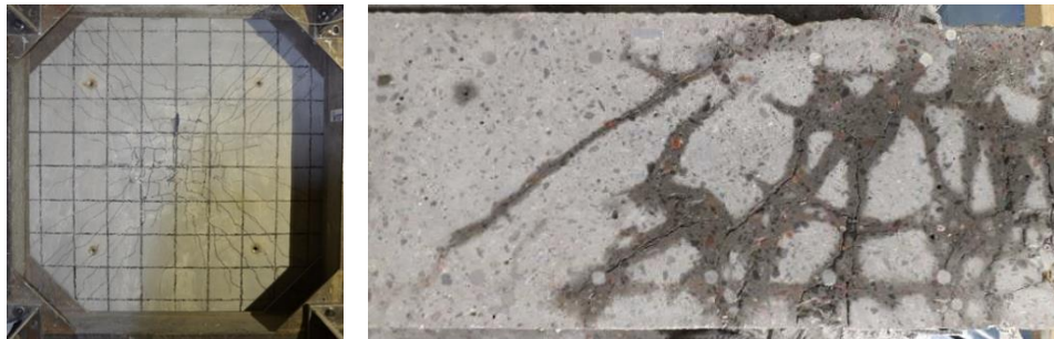
Figure 6. Test X12: Rear side (left) und vertical section of test slab (right).
