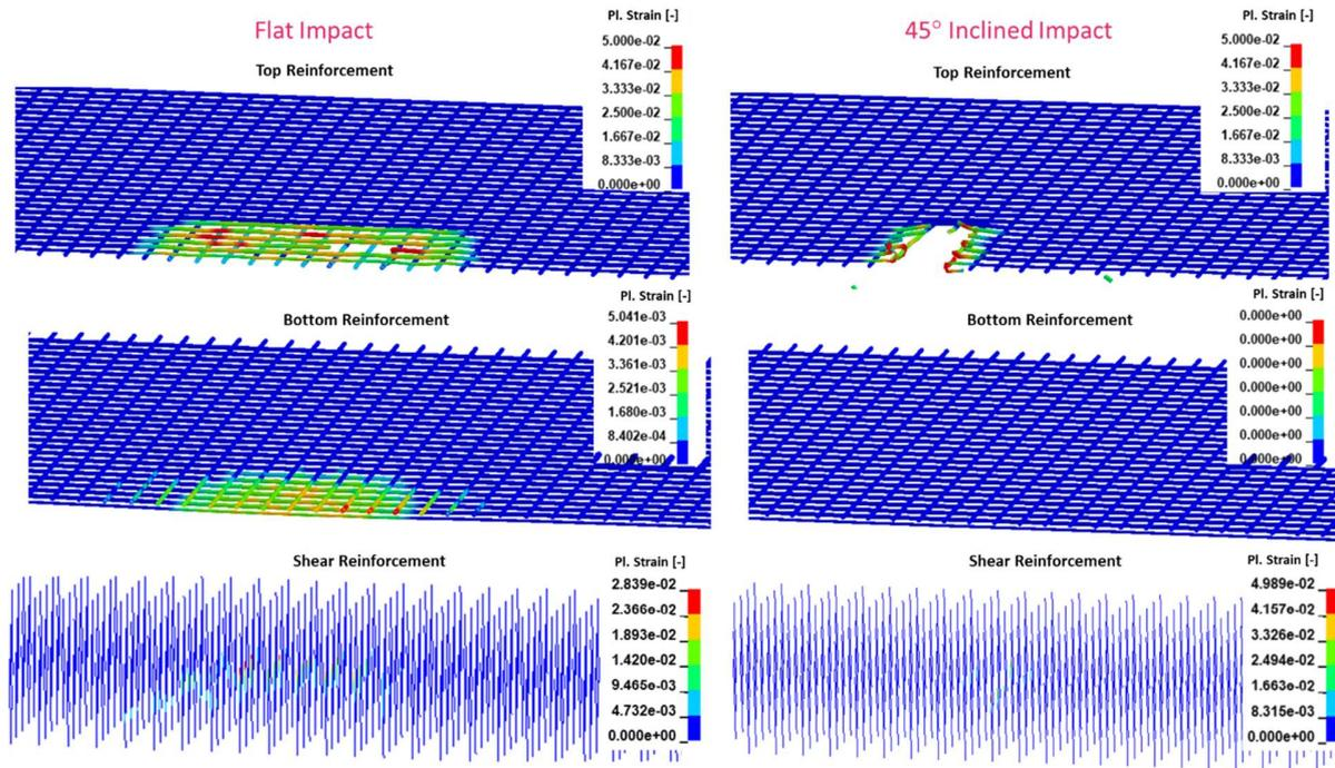
Figure 7. Maximum calculated strains of the bending reinforcement
