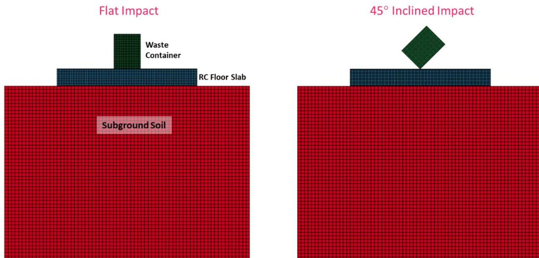
Figure 1. Finite element model geometry for a flat impact (left), and for an impact with 45° angle (right)
