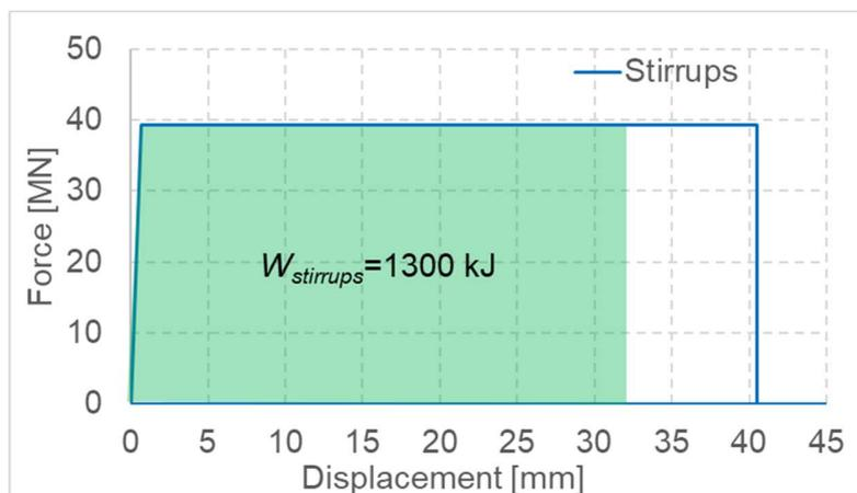
Figure 9. Deformation energy of the shear reinforcement
