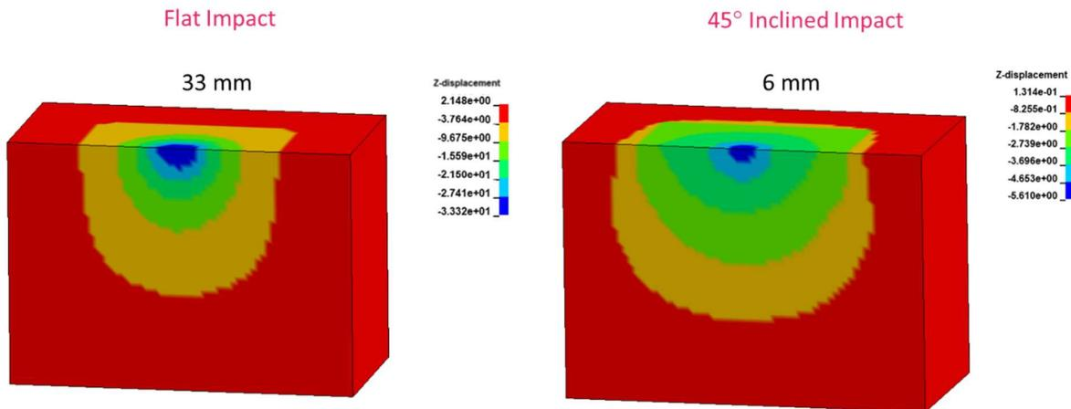
Figure 8. Maximum displacement in the subground soil
