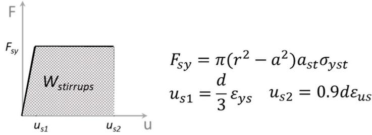
Figure 4. Energy absorption of stirrups
