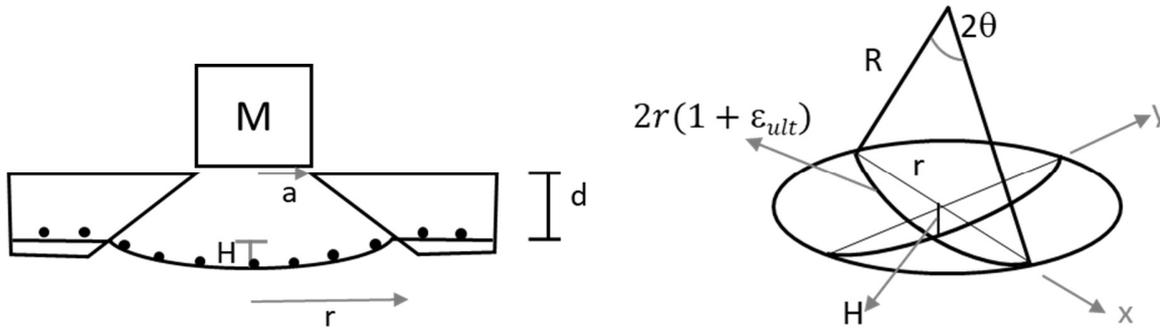
Figure 3. Considered punching cone (left) and the geometry of the mathematical model (right)
