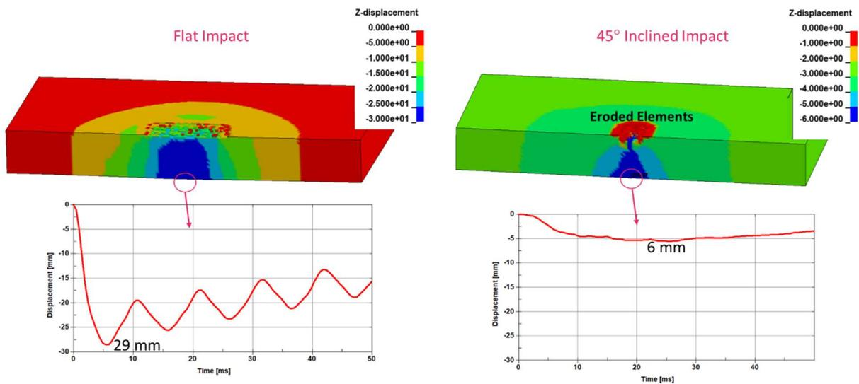
Figure 6. Time histories of the maximum displacements in the RC floor slab
