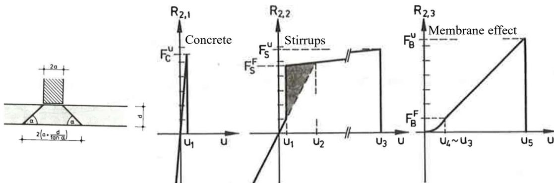
Figure 2. Spring properties for the punching cone according to Schlüter 1987
