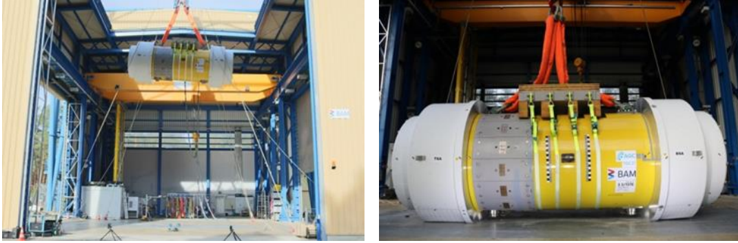
Figure 5. Test specimen ready for the 9.3-m free drop test and after the 9.3-m drop test (source: BAM)
