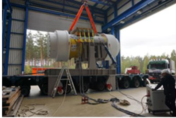
Figure 4: Positioning of the test specimen into a horizontal 4° drop orientation with a handling device
