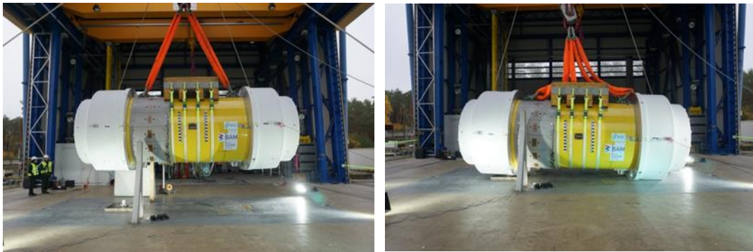
Figure 6. Test specimen ready for the 1-m puncture bar drop test and after the 1-m puncture bar drop test (source: BAM)
