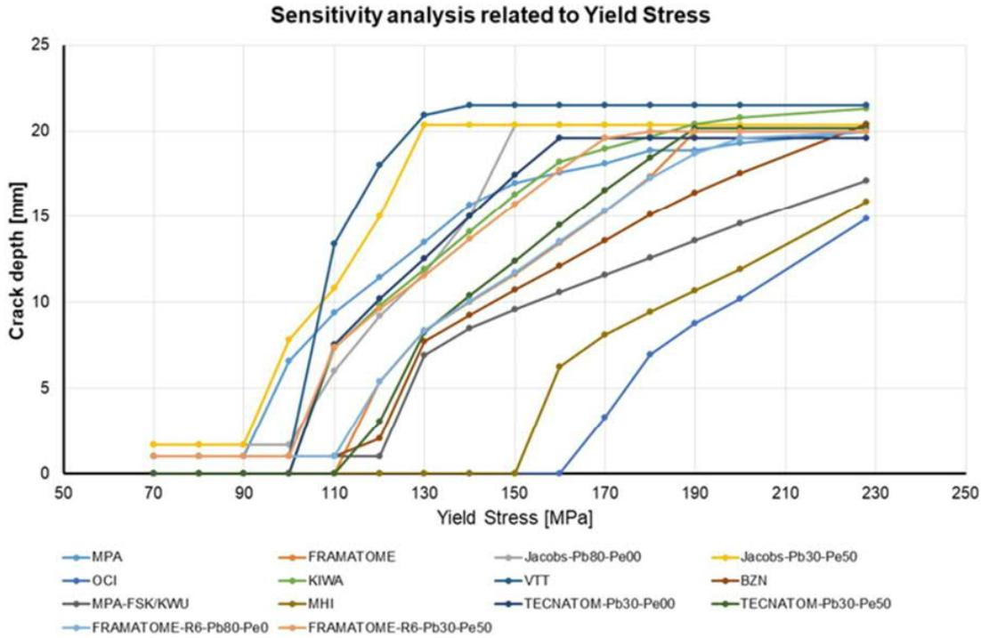
Figure 4. Influence of Yield Stress on Surface Defect Limit State.
