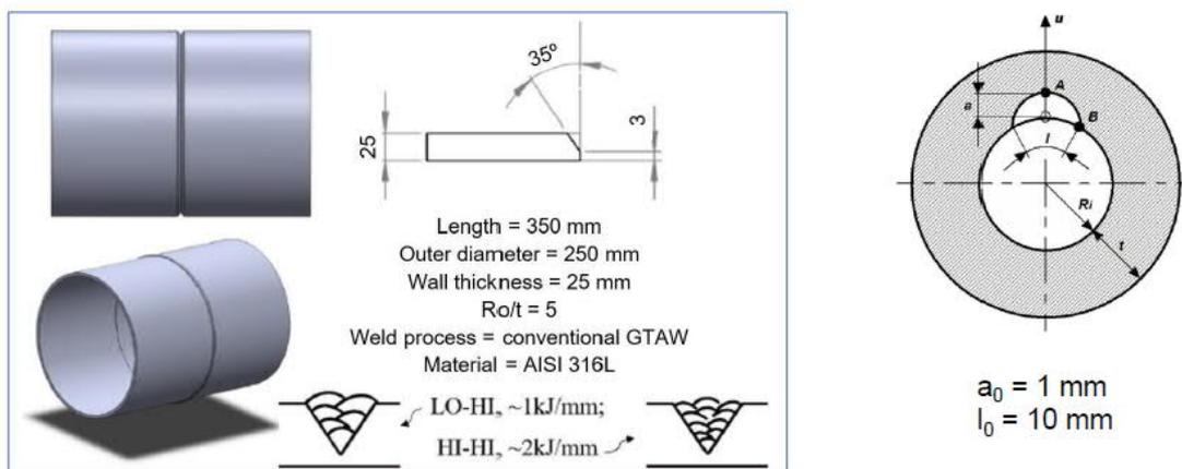
Figure 2. Weld and Pipe Geometry for PBC-6 Case
