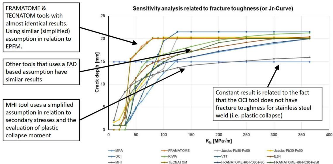
Figure 3. Influence of Fracture Toughness on Surface Defect Limit State.
