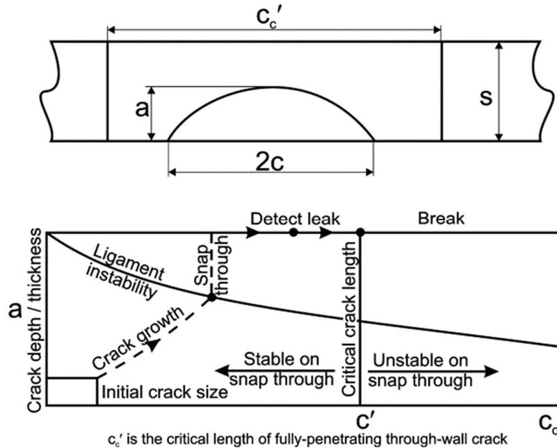
Figure 1. LbB Diagram of the various Crack Growth Stages (from R6 [EDF Energy 2019])
