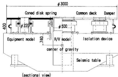
Figure 3. Vertical isolation system model.
