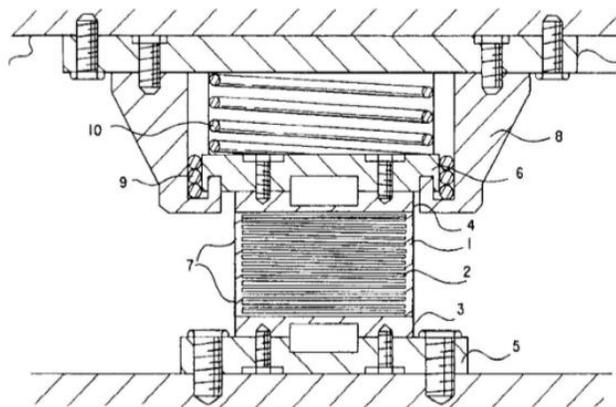
Figure 1. Schematic Drawing of 3-D Seismic Isolation Device.
