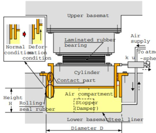
Figure 2. The 3-D base isolation device with rolling sealed air spring.
