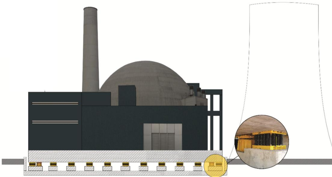
Figure 1. 3-D Base Control System below NPP building.
