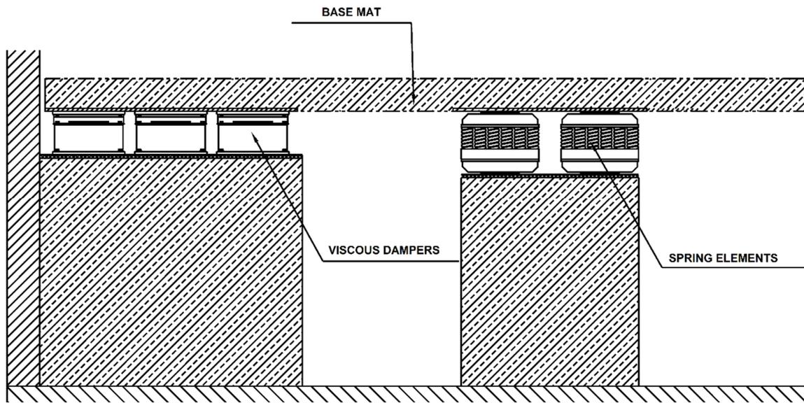
Figure 2. Devices below the floor slab of the building.
