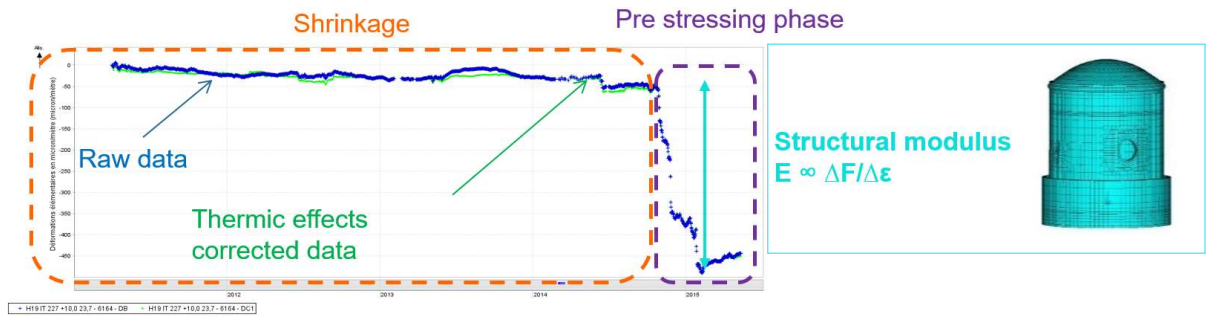
Figure 3: Example of strain monitoring during construction
