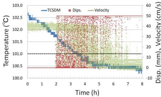
Figure 9. Relationship between TCSDM, displacement, and flow velocity (Case 2)
