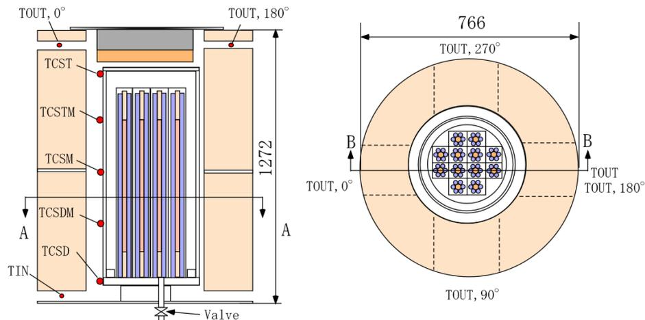
Fig. 2. 1/4.5-scale cask model. TIN, air inlet temperature; TOUT, outlet temperature; TCSDM, canister surface temperature at mid-point of lower portion of the canister.
