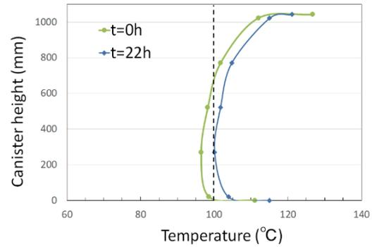
Fig. 6. Canister surface temperature (Case 1)
