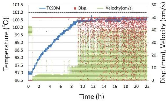
Fig. 5. Relationship between TCSDM, displacement, and flow velocity (Case 1)
