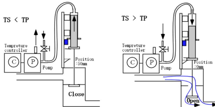
Fig. 1. Flow adjustment device
