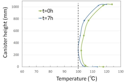
Figure 10. Canister surface temperature (Case 2)
