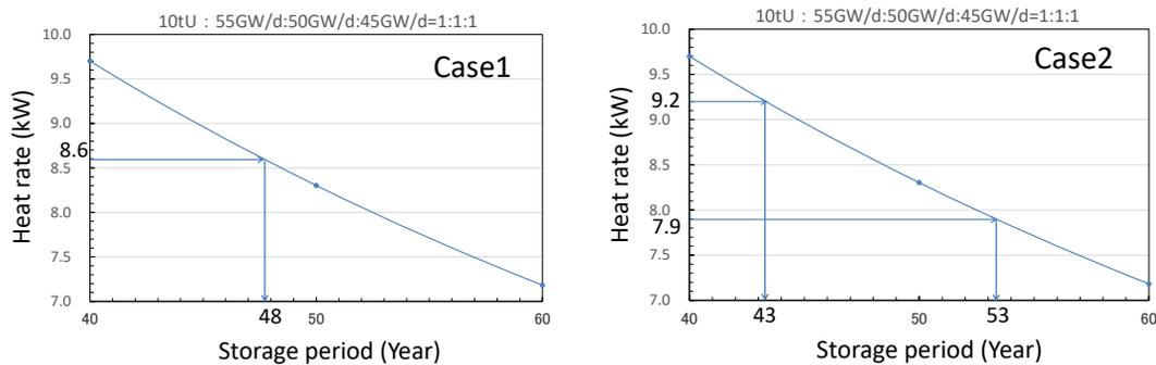
Fig. 4. Relation between storage period and decay heat rate in an actual canister.
