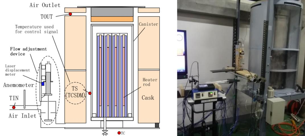
Fig. 3. Installation drawing and photograph of the air inlet of the flow adjustment device. TIN, TOUT, and TCSDM (TS) are defined in Fig. 2.
