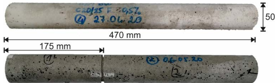
Figure 2. Specimens for the spalling tests
